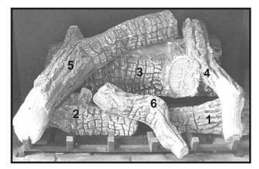
**STEP 7:** (SRV2057-725): Place log 6 on log 2 as shown. The left end of log 6 should touch the upper knot of log 2. The right end of log 6 should rest on the grate bar, centered between tine 4 and 5. NOTE: The front faces (C) of log 6 and 2 should be on the same plane. This is key in avoiding flame impingement.
